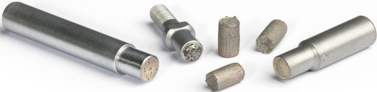
Diamond grit impregnated dressers have been developed from multi-point dressers. In contrast to the latter they are manufactured from crushed diamond grit rather than a larger number of small natural diamonds. The advantage of the diamond impregnated dresser lies in its exceptional sharpness, which results from sharp edges and points of the broken diamond grit.
